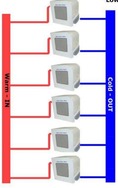
3/4" Pipe = 11 Gallon Per Minute for 1 Dome Heater
